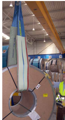
Clip on sleeve SC for SpanSet heavy-load Powersling CS as per sketch 1
