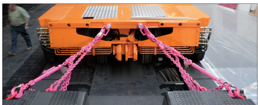
Four bearing strands by VIP lashing chains with special balancer rolls
